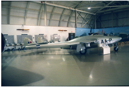
The de Havilland Vampire was Unusual in that it was a Plywood-Aluminum Composite
